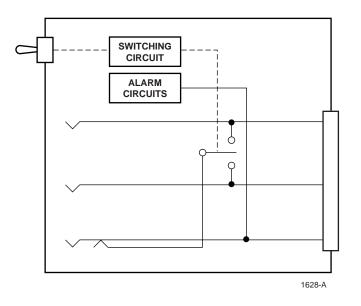
Figure 4-1. PSM-812001 Module Block Diagram
